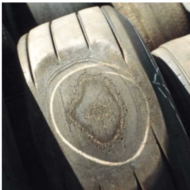
Locked wheel tire flat spot
