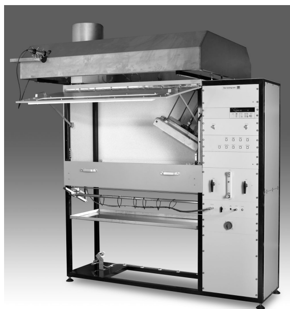
FIGURE 4.1(a) Flooring Radiant Panel Test Apparatus.
