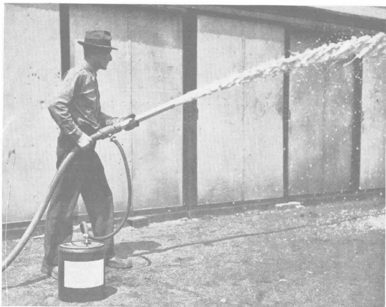
Fig. A-1155. Air Foam Playpipe.
