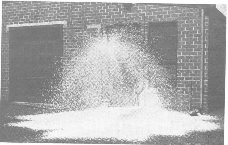
Fig. A-200B. Overhead Air Foam Spray.
