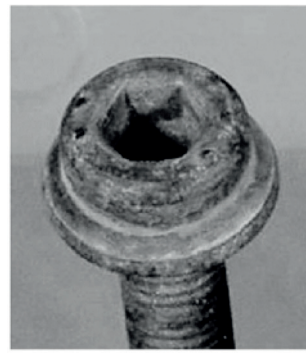
b) Zinc-nickel after 1 000 h NSS testing
